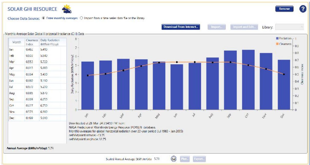
Figure 4-6: Solar GHI resource for Matuwamba site, Mzimba
