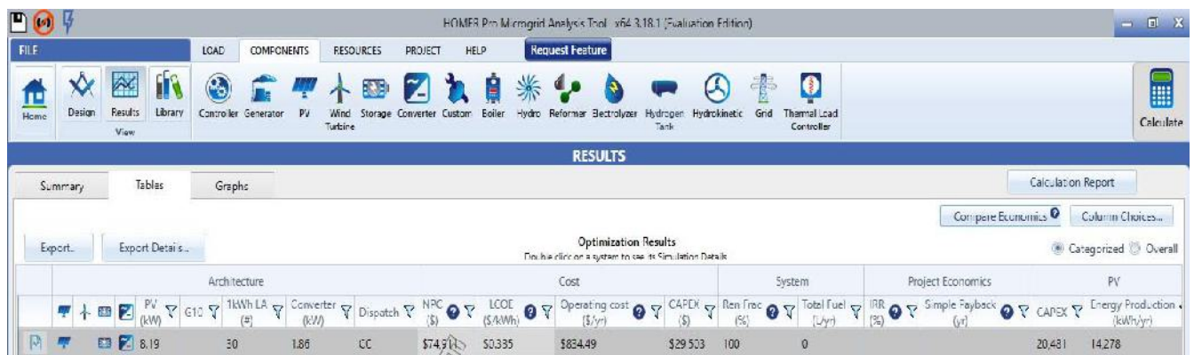
Figure 4-5: Simulation results for Luviri solar mini-grid
